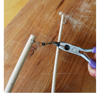
11. Connect the wires on the dowels by looping a swivel over the ends of the wires and crimping with the pliers.
