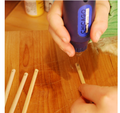
8. Drill holes in all points that will be connected with a swivel.
